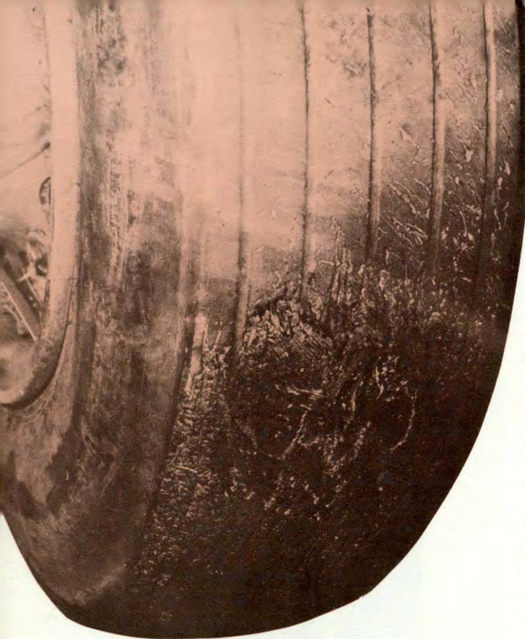
Right main tire with reverted rubber skid mark.
